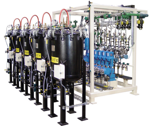
Blending Equipment : 4 - formulations automatically blended in a random order.
