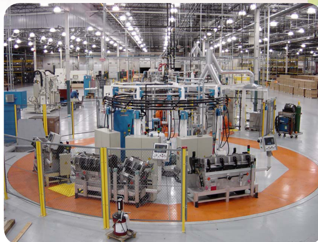
Complete Foam Processing Line for the Mercedes R-Class Instrument Panel
